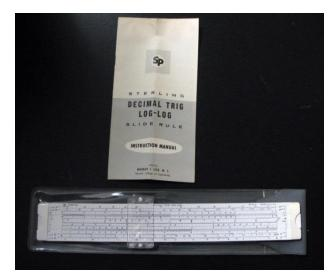
Slide Rule – Pilots and astronauts used slide rules to make calculations before there were computers. Slide rules help with multiplication, division, and calculus equations. This slide rule comes in a case with a manual.
