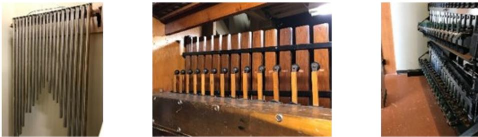
Others make up **toy counters** and include **drums, cymbals, slide whistles, doorbells, and other special effects**. All of these are operated from the console through mechanisms very similar to the regular windchests.
