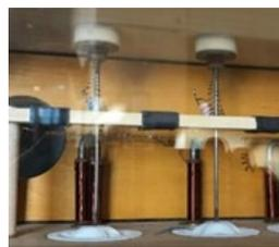
The regulated air is then delivered to an air-tight **windchest**. The **pipes** sit on individual holes in the top side of the windchest, and each hole is fitted with a **valve**. The valve is controlled by an **electromagnet** that is wired to the keys in the console. When a key is pressed, it closes a circuit that makes the valve open, and the air inside the windchest escapes through the hole and into the pipe, making it play.
