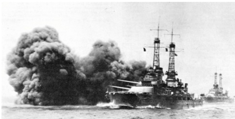
The USS Oklahoma demonstrating its firepower during gunnery practice. Each shell fired by her 14-inch guns required 420 pounds of gunpowder (image 80-G-1023157, courtesy of Naval Heritage & History Command).
