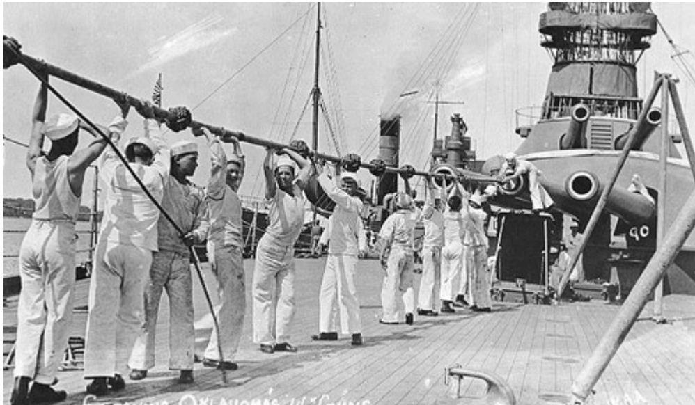
Sailors moving a 14-inch shell around the deck, by hand (image courtesy of the Library of Congress).
