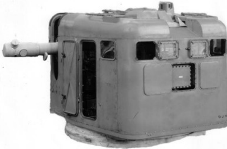
This is a Mark 19 Gun Director. The USS Oklahoma had one just like this. The knob sticking out from the box is the gun director's rangefinder (OHS Collections).
