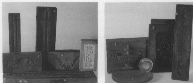
Figure 8. Several historic and reproduction compo molds are shown to underscore the variety of materials used to make them: 1. applewood mold 2. pearwood mold 3. boxwood mold encased in beech 4. boxwood mold 5. sulfur mold encased in maple 6. pewter mold encased in pine and oak 7. positive pattern for pitch mold carved in pearwood 8. pitch mold encased in oak 9. composition mold encased in maple 10. epoxy and polyester molds reinforced with glass fabric. Photos: Jonathan Thornton.
