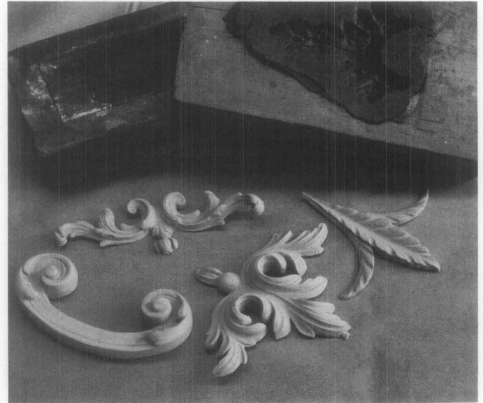
Figure 30. Based on documentary and physical evidence, missing composition ornament was accurately re-created for the Miles-Brewton House, Charleston, South Carolina. First (a) the conservator used molds to fabricate ornament in small pieces and lengths; and (b) the new ornament was attached to thin birch plywood backing with glue and brads to create larger sections. These sections were then fastened to the original paneling with stainless steel screws. Photos: Jonathan Thornton
