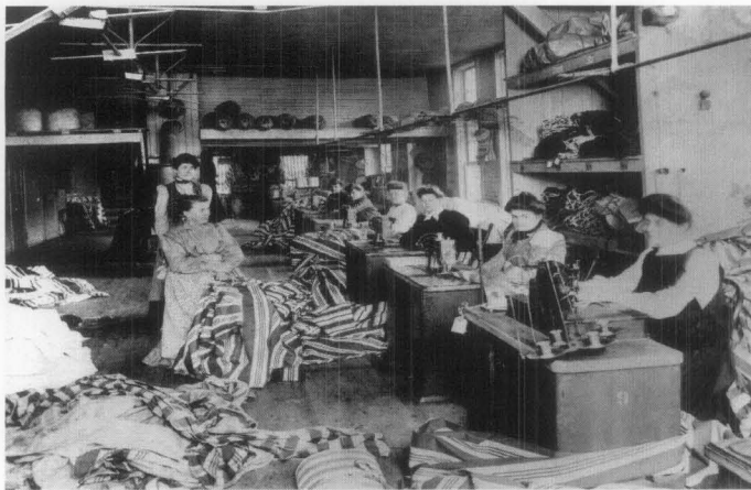
Figure 4. This 1892 photo shows the canvas sewing room of a large awning manufacturer. The wide variety of custom sizes and shapes, and the natural shrinkage of canvas demanded considerable skill in measuring, cutting and sewing. Photo: The Astrup Company.
